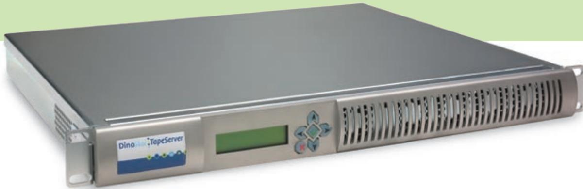
**DinoStor TapeServers bridge SCSI and FC tape devices to Gigabit Ethernet so that NDMP-capable NAS servers can share tape devices via Ethernet. By optionally encrypting the backup data, TapeServers also prevent data theft if tapes are lost.**
